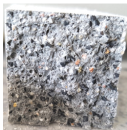
Fig. 4. 4x4 cm fracture of the GK-D cement mortar beam after bending strength test with visible black SBR-D rubber granules
