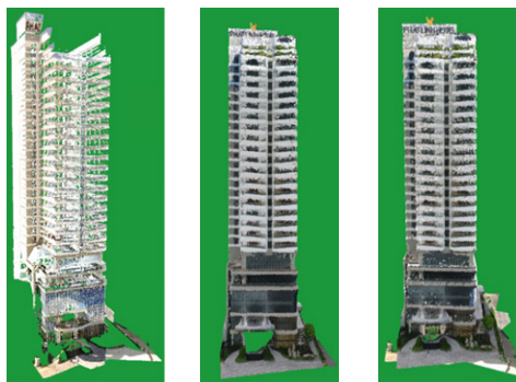
Fig. 10. High building's TLS point cloud after noise filtering (a), High building's UAV point cloud after noise filtering (b), High building's UAV and TLS point cloud after precision matching (c)
