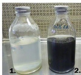
Fig. 1. Formation of black precipitates FeS (1 – abiotic control, 2 – at presence of SRB)
