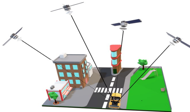
Fig. 2. Mobile laser scanning system using GNSS-IMU positioning for direct georeferencing of received data
