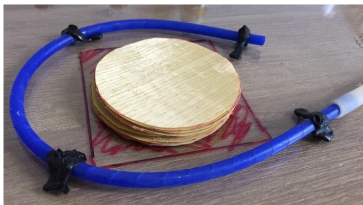
Fig. 3. The process of making a sample for testing
