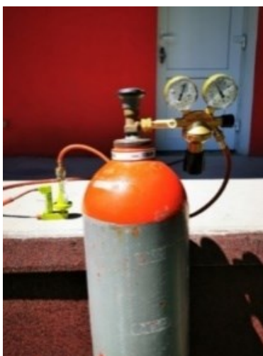
Fig. 1. Introduction gas system into the enclosure
