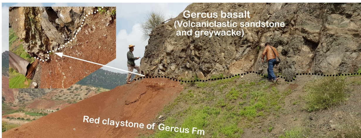
Fig. 2. The contact between Gercus (Duhok) Basalt and Gercus Formation is sharp and barren of contact metamorphism, chilled border, and mineralization. This indicates cold emplacement of claim basalt (present greywackes). This condition is true for all igneous bodies and dykes in the Mawat, Bulfat and Penjween claimed Ophiolite Complexes.
