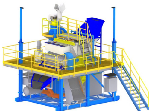
Rys. 8. Mobilny system wzbogacania odpadów Fig. 8. Mobile waste enrichment system
