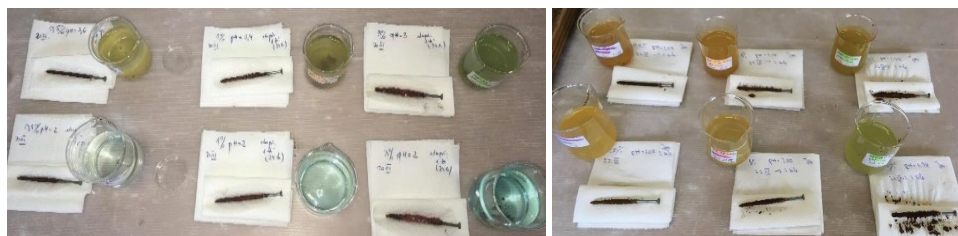
Fig. 2. Samples with the amount of copper deposited on the iron, from different days of the experiment
