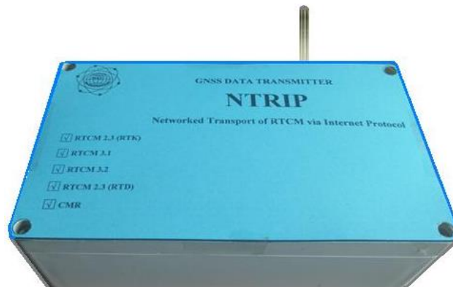
Fig. 4. GNSS data transmitter by NTRIP.
