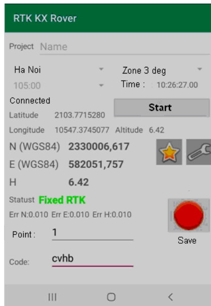
Fig. 8. Interface of RTK KX Rover software installed in a smartphone.
