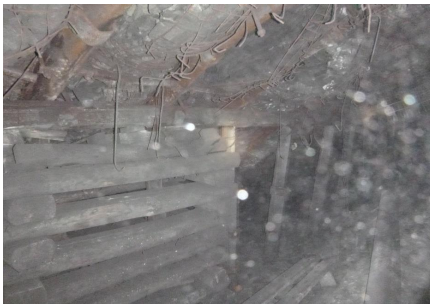
Fig. 13. View on the monitor wood crib behind the longwall face PW-1.
