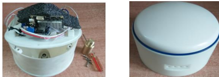
Fig. 7. Developed GNSS RTK receivers KX20-R: incomplete (left) and completed (right)
