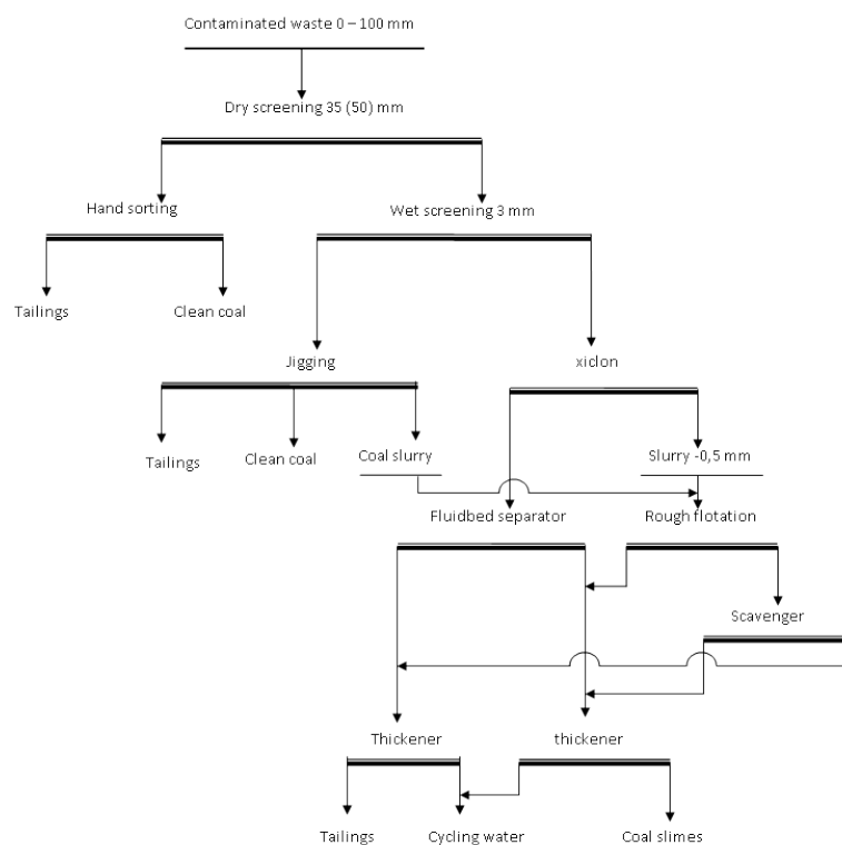
Fig 2. Washing flowsheet for contaminated waste containing size fraction 0 - 3 mm with the ash content over 40%.
