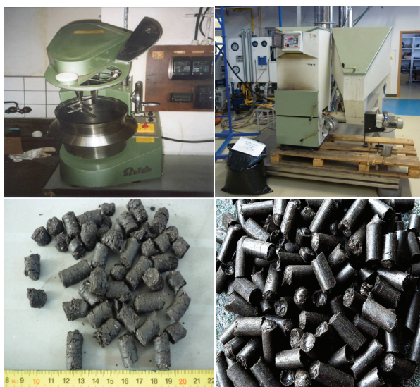
Fig. 3. Photographic evidence – alternative multicomponent fuel based on fuels treated on the device for physical waste treatment as per EP 2388068 “Device for Physical Waste treatment” – homogenisation of components at the stage before granulation in cooperation with Czech Brown Coal Research Institute, Inc. (VÚHU a.s.) in Most, combustion testing on a certified testing equipment at VŠB – Technical University in Ostrava, examples of final granulated multicomponent solid alternative fuel
