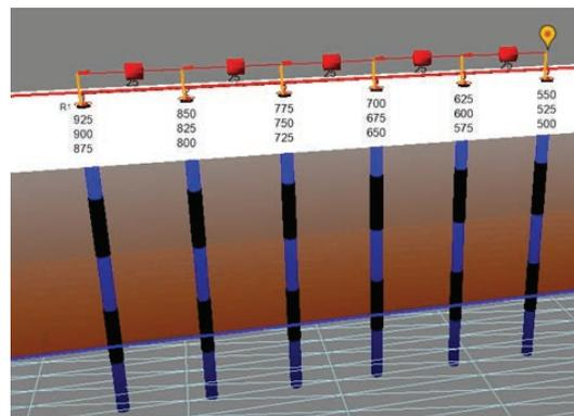
Fig. 1. The blasting series designed in the O-Pitblast software
