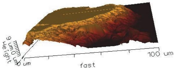
Fig. 7a. AMD immersed part of concrete sample
