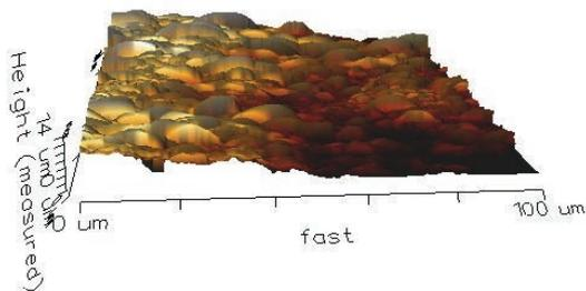
Fig. 8b. Non immersed part of concrete sample taken out from DW
