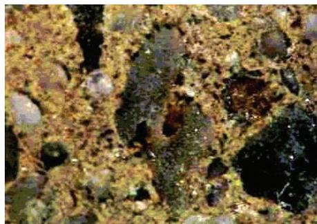
Fig. 5b. Considerable biodeterioration of concrete sample surface after 90 days. Magnification of image 20 x 4,5
