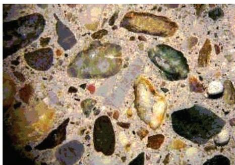
Fig. 5a. Smooth surface filling among aggregates before experiment Magnification of image 20 x 4,5
