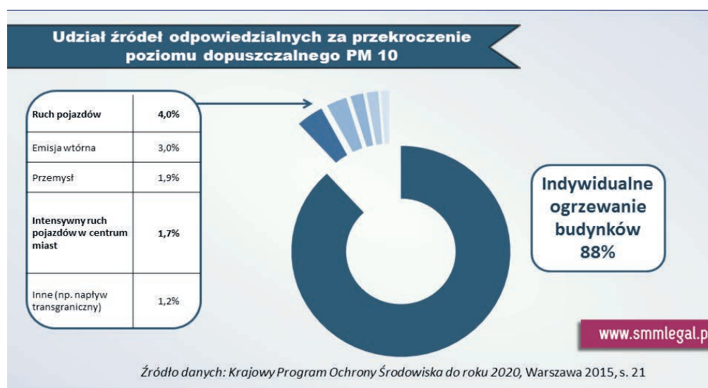
Fig. 2. The participation of sources responsible for transgression of acceptable level of the PM 10 dust in Poland. Source: [4]
