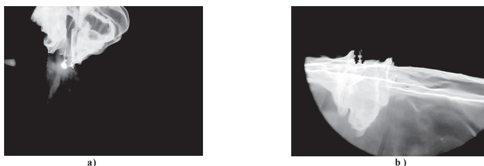
Fig. 5. Illustrative photo for 73.0 vol. % of H 2 /CO/CO 2 /O 2 /N 2 mixture with 27.0 vol. % of air at T 0 = 298 K: a) early stage of explosion initiation; b) end of ignition process.
