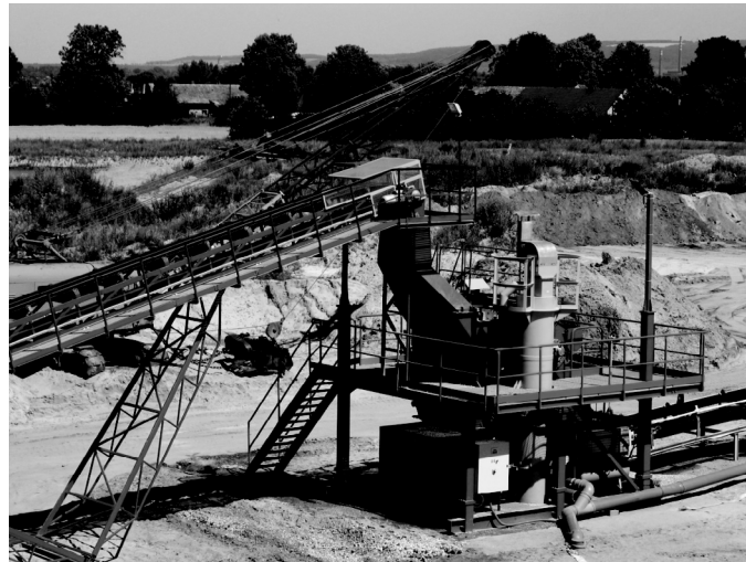
Fig. 6 Pulsated jig K-100 in Januszkowice preparation plant
