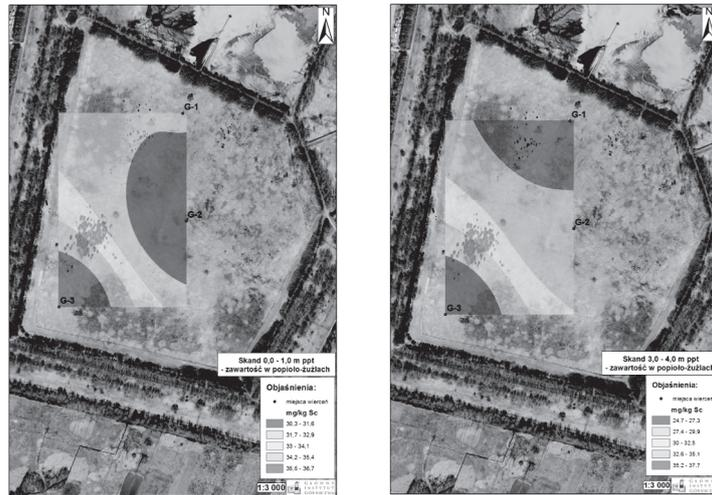
Fig. 5. Map of horizontal distribution of scandium content a) in the 0.0 to 1.0 m bgl layer, b) in the 3.0 to 4.0 m bgl layer
