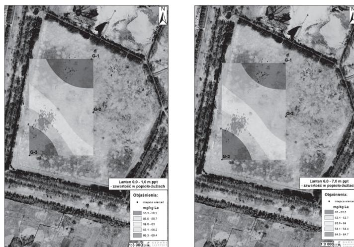
Fig. 7. Map of horizontal distribution of lanthanum content a) in the 0.0 to 1.0 m bgl layer, b) in the 6.0 to 7.0 m bgl layer
