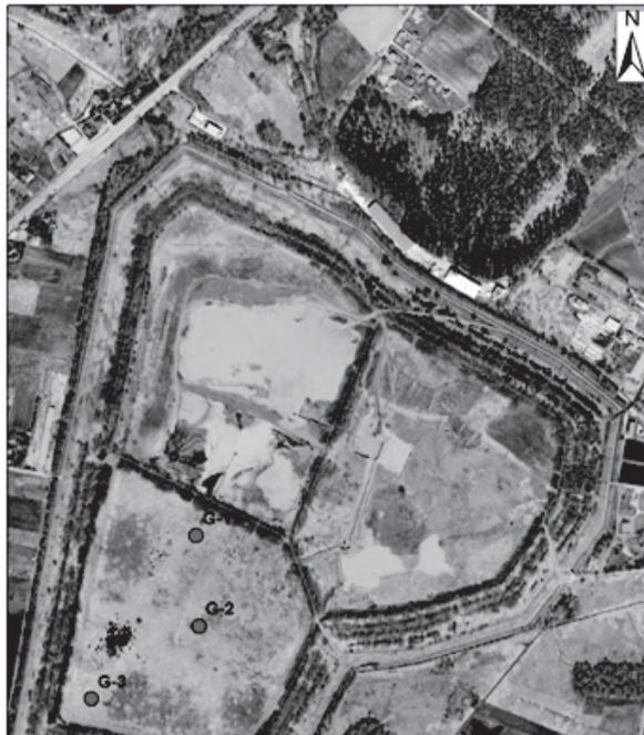
Fig. 3. The location of boreholes and sampling spots in the “Gardawice” landfill
