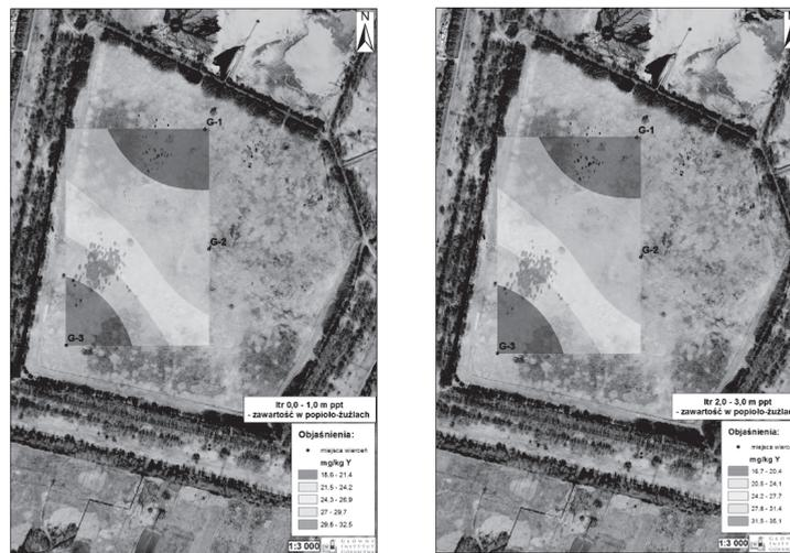
Fig. 6. Map of horizontal distribution of yttrium content a) in the 0.0 to 1.0 m bgl layer, b) in the 2.0 to 3.0 m bgl layer
