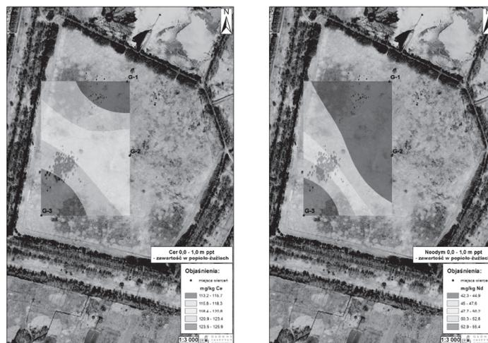
Fig. 8. Map of horizontal distribution a) of cerium content in the 0.0 to 1.0 m bgl layer, b) of neodymium content in the 0.0 to 1.0 m bgl layer
