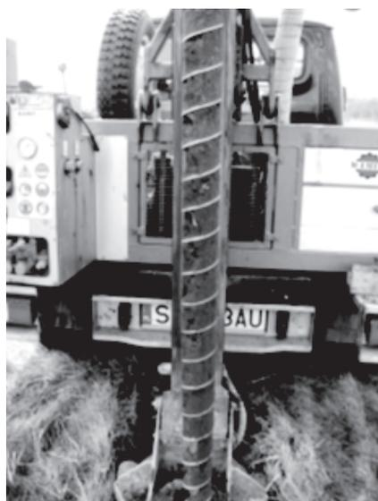
Fig. 4. The auger filled with an ash-slag mix
