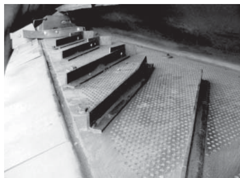
Figure 1 and 2. Separating deck of the FGX-1 air concentrating table [source: Photo by Wojciech Sobko]
