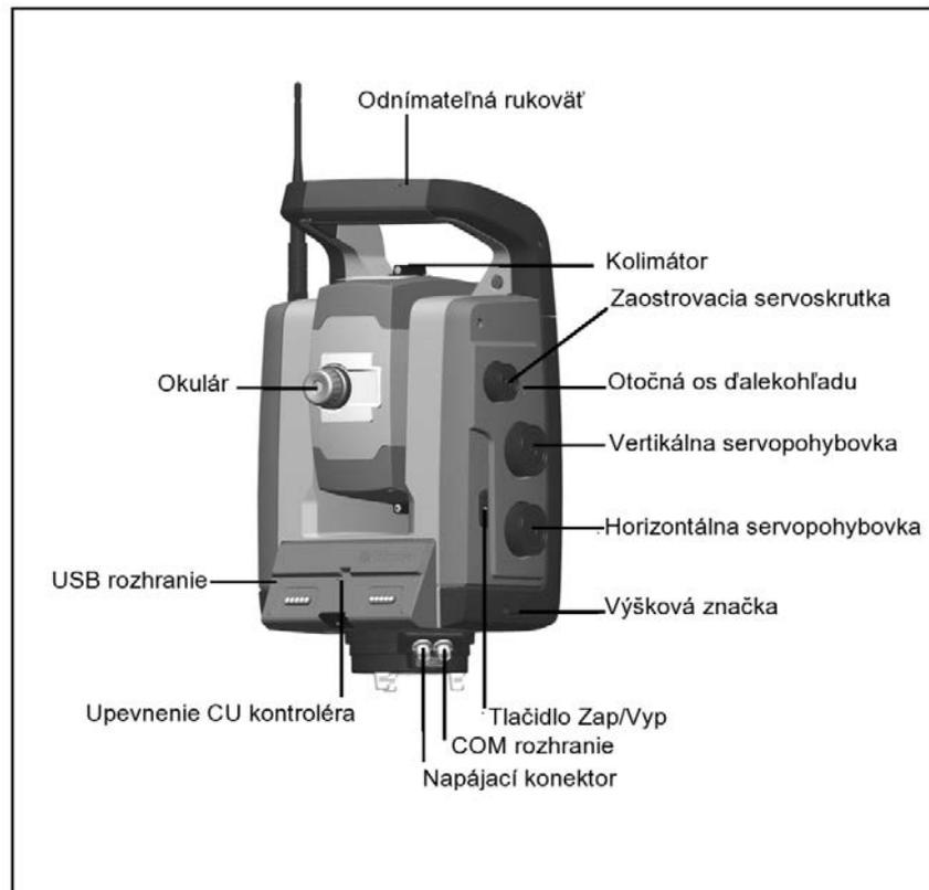
Fig. 1.1. The basic controls and the design features (the view from the position of the operator)
