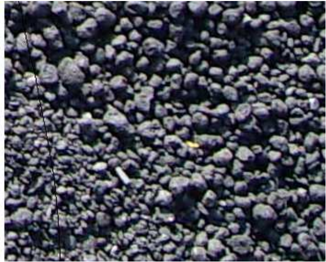
Fig. 2 Granulated coal slimes with the content of FBC ash
